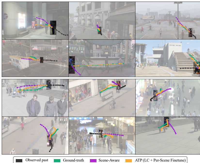
Fig. 3: Qualitative results on MotSynth (top; synthetic) and MOT and WildTrack (bottom; real). These examples show scenarios where our LC + per-scene finetune ATP method (orange) outperforms the scene-aware baseline (purple). In several MOTSynth examples, the baseline predicts the pedestrian floats into the air (top row), while our method has gained awareness of where the 3D ground plane lies in the 2D image. We also note that patterns of behaviour such as walking on the sidewalk instead of into the road (second row left) and walking up the traversable portion of stairs (second row right) are captured. On real data, we observe similar awareness of the ground plane and obstacles, as well as a better understanding of nuanced human behavior patterns such as crossing diagonally across a plaza.
